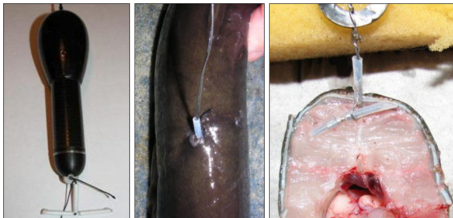
Figure 6 Photos of the Økland-Westerberg anchor implant method used to attach pop-up satellite archival transmitters to European silver eel.
