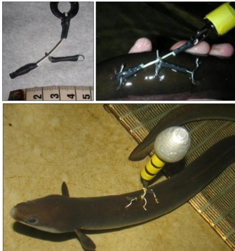
Figure 5 Photos of the Westerberg method used to attach pop-up satellite archival transmitters to European silver eel.
