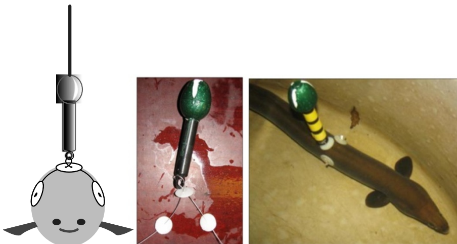
Figure 4 Illustration and photos of the Jellyman and Tsukamoto tagging method used to attach pop-up satellite archival transmitters to European silver eel. The method is slightly modified from the tagging method described by Jellyman and Tsukamoto [11-13].
