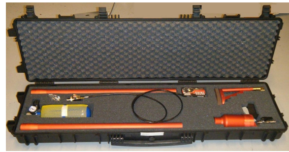
Fig. 4 Standard ARTS (ARTS-S) kit with 2 barrels (840 mm), one small pressure bottle with a reduction valve and a 2,5 m long pressure hose, one aiming sight (Riflescope ZOS), and the ARTS pressure chamber (lower right), a quick shoulder shaft and a quick connector to the pressure tank. Photo by Tom Are Mathisen. Rev2
