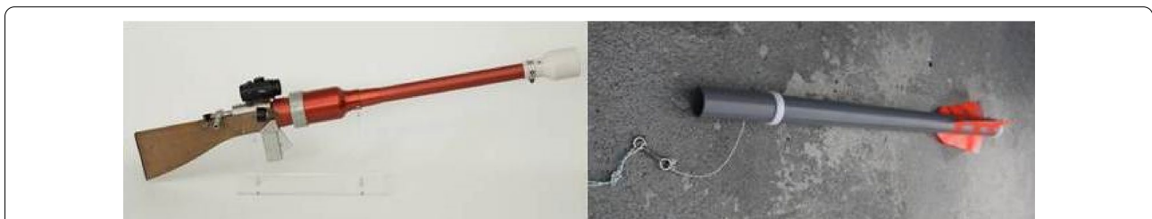
Fig. 2 Early prototype of the ARTS (1998), left panel and the ARTSCarrier, with a Galvanic Time Release line (1998), right panel. Photo by Tom Are Mathisen and Lars Kleivane
