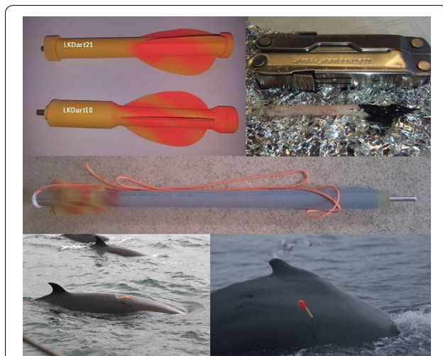
Fig. 10 LKDart21 and LKDart10 (upper panel left). Upper panel right shows a blubber sample collected with a Finn Larsen biopsy tip, 80 mm long. Middle panel show the tethered setup for the LKDart, the LKTDart, while lower panels demonstrate biopsy sampling of a northern bottlenose (left) whale and humpback whale (right), using the LKDart10. Photo by Lars Kleivane and Saana Isojunno
