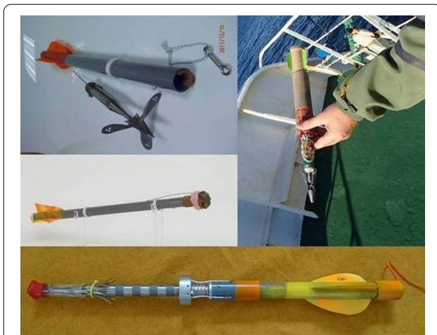
Fig. 5 Use of different ARTS-Carriers when deploying satellite tags, shown in upper left panel (ARTSC) with GTR release line, a satellite tag from Wildlife Computers (SPOT5 mold 177) and anchor from IMR (Institute of Marine Research, Norway); upper right panel (ARTSC1) a setup with the same satellite tag but with different carrier design, with an anchor from NRISFS (National Research Institute of Fisheries Science, Japan); in middle left panel the ARTSLC for the Wildlife Computer LIMPET Tag SPLASH 292, anchors from Wildlife Computers not illustrated. In lower panel the ARTSTBC, a tethered system including a biopsy tip, for Wildlife Computers tags SPOT303/SPLASH302. Photos by Lars Kleivane
