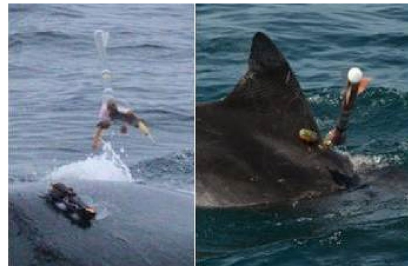
Fig. 11 Left panel the Mixed-DTAG deployed to a humpback whale. Right panel a LIMPET tag (WC, SPLASH 292) deployed to a bottlenose dolphin ( Tursiops truncatus ). Both simultaneously collecting a biopsy sample. Photo by Christopher Hinchcliffe and Leonardo Wedekin
