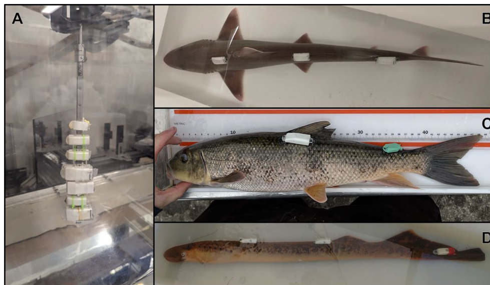
Fig. 1 Pictures of multiple tags during each experimental set up. During robotic experiments (A) multiple tags were affixed to a rigid metal rod and simultaneously moved sinusoidally in heave and pitch to provide known a input movement pattern to all tags using a robotic flapping mechanism. Multiple tags were additionally attached along the body onto live animals including a smooth dogfish (B), white sucker (C) and sea lamprey (D)
